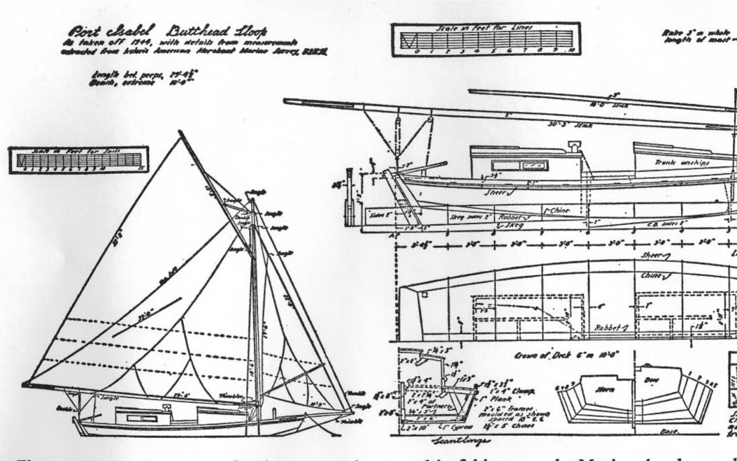
Fig. 121. Texas scow sloop fitted as a camp boat, used in fishing near the Mexican border on the scows are without dead rise. The boats range from 26 to 35 feet in length, 10 to 12 feet beam with the head sprung forward.
